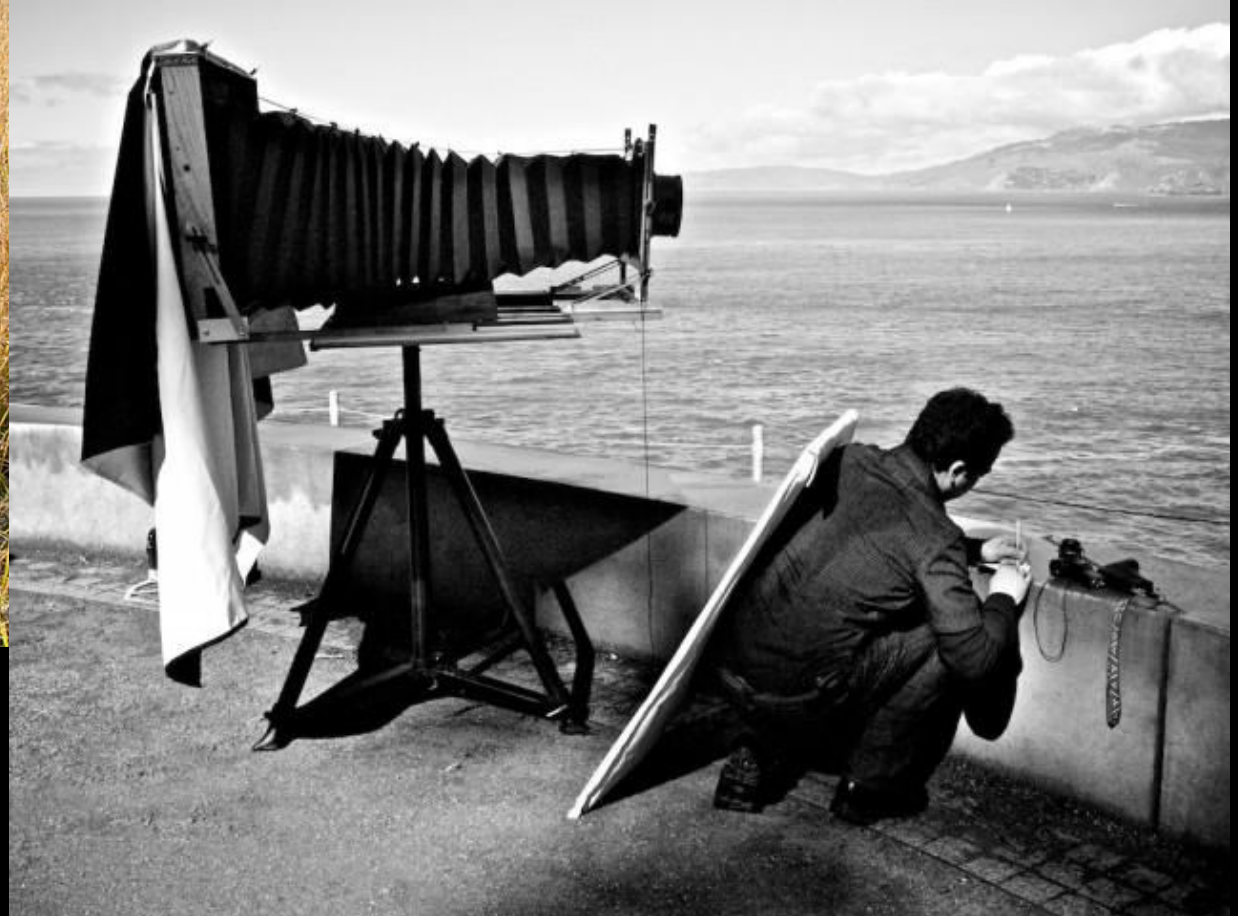
San Francisco photographer Darren Samuelson built his own six foot-long ultra large format camera that uses 14" X 36" X-ray film negatives.
